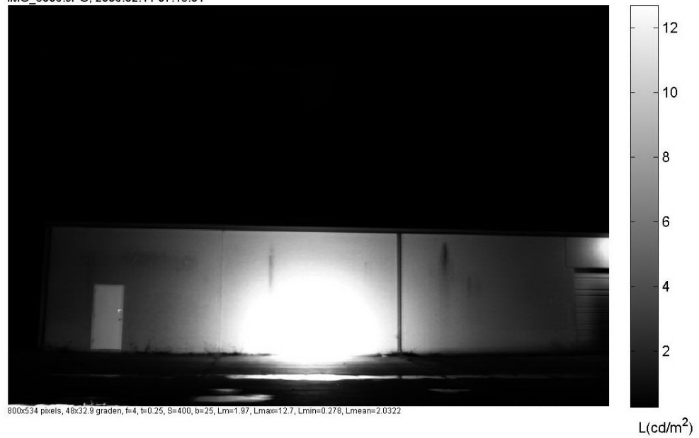
Figure 21 The luminance of the Carbon Arclight projected onto a wall at a distance of 100 meter.
