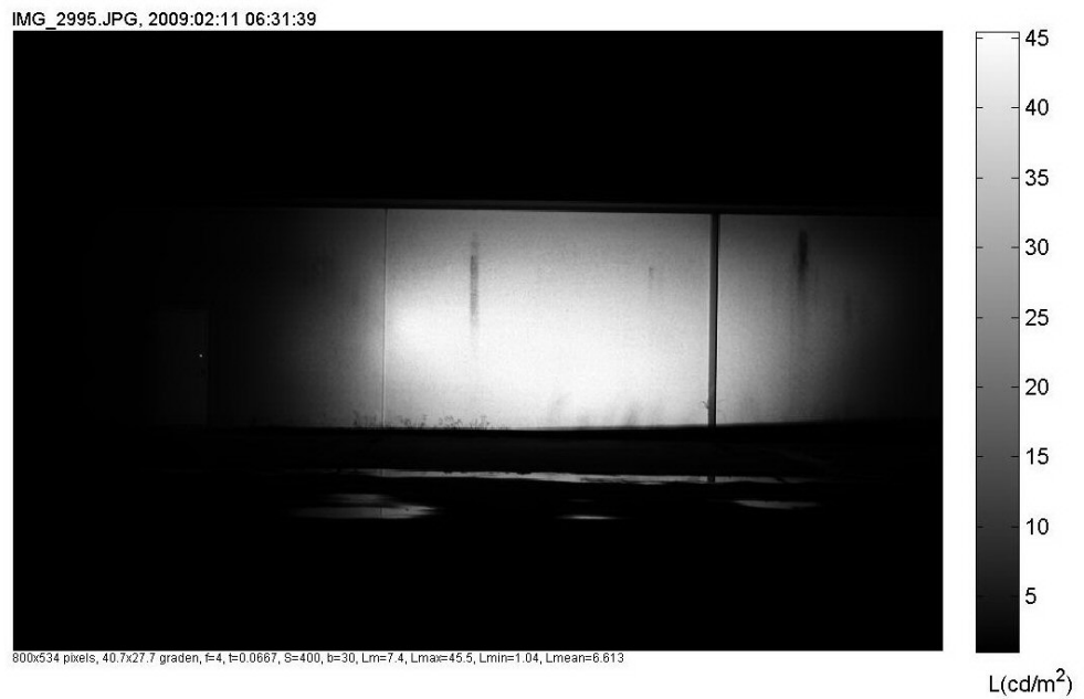
Figure 23 The luminance of the Prolight projected onto a wall at a distance of 100 meter.
