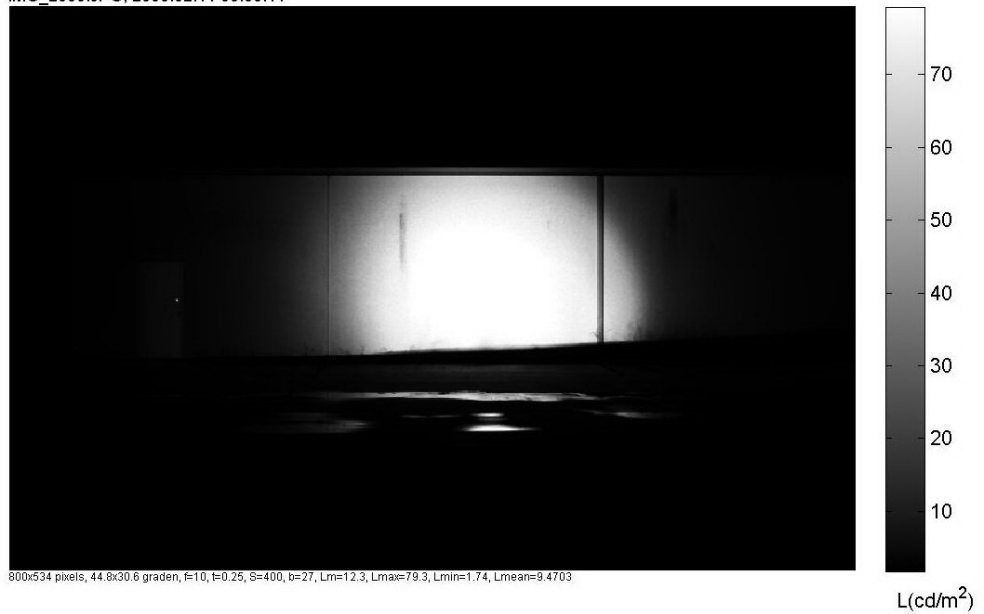
Figure 19 The luminance of the Skytracker projected onto a wall at a distance of 100 meter.
