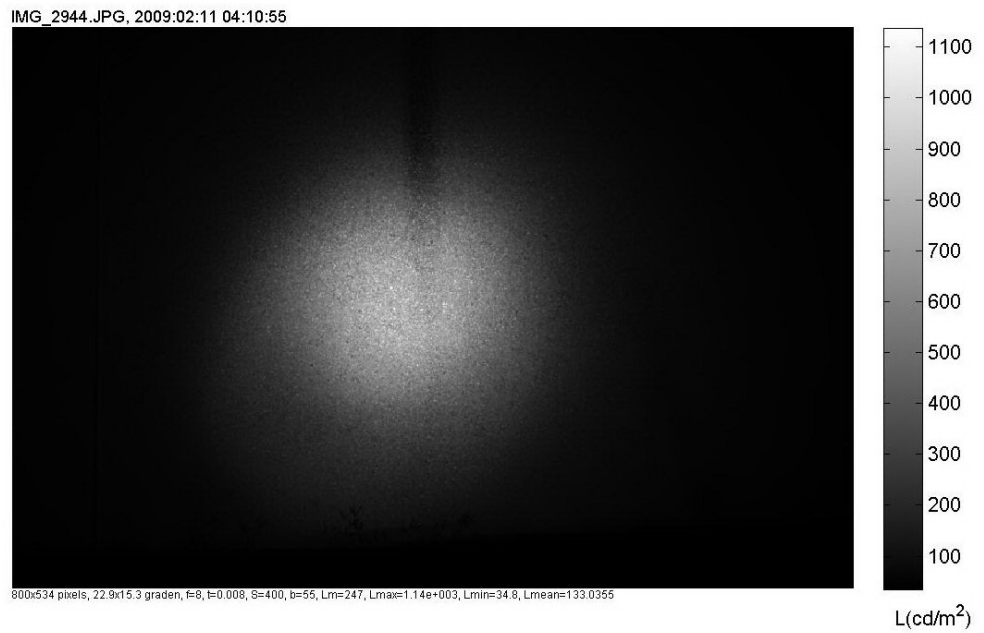
Figure 25 The luminance of the 2k Xenon Light projected onto a wall at a distance of 100 meter.
