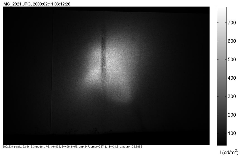
Figure 15 The luminance at the wall when light from the handheld Arlight is projected from a distance of 100 meter.
