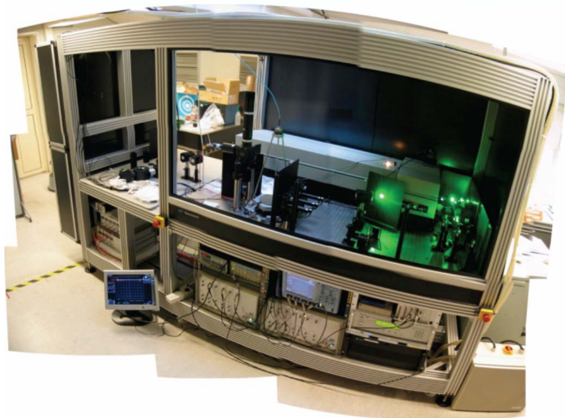
Figure 45 Complete system layout (source: RIVM). The frame containing the LIDAR system is in the middle of a room in a 20 ft container, so that it can be accessed from all sides for maintenance. Service elements such as large power supplies are in a separate compartment.
