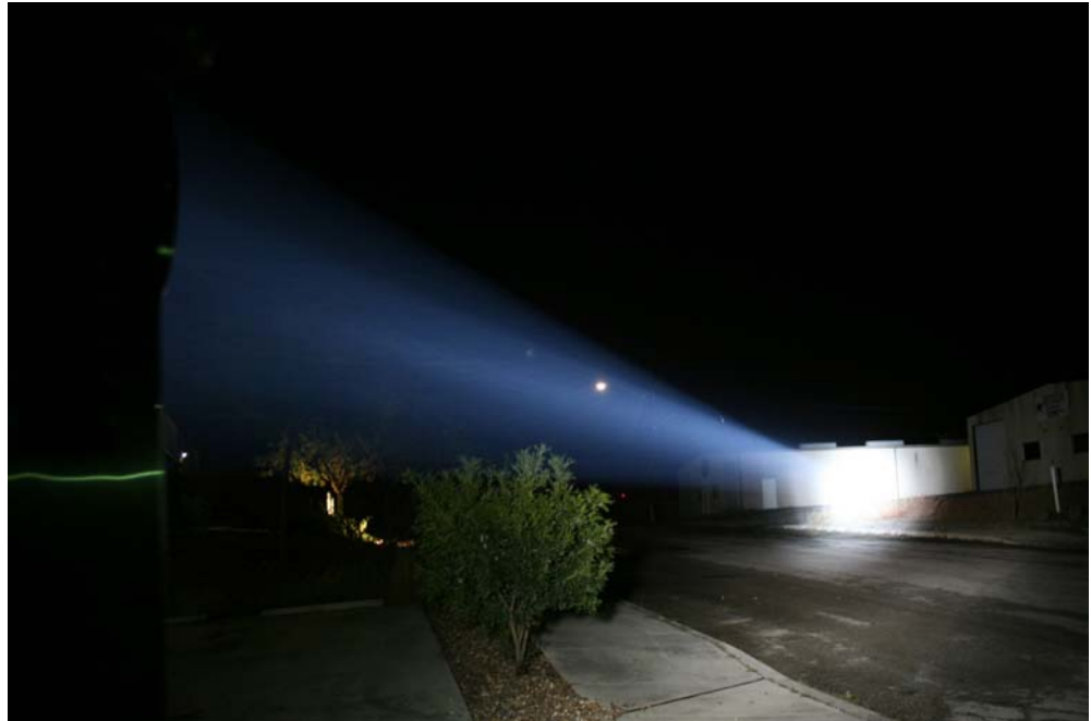
Figure 12 Searchlight projected onto a wall at a distance of 100 meters.
