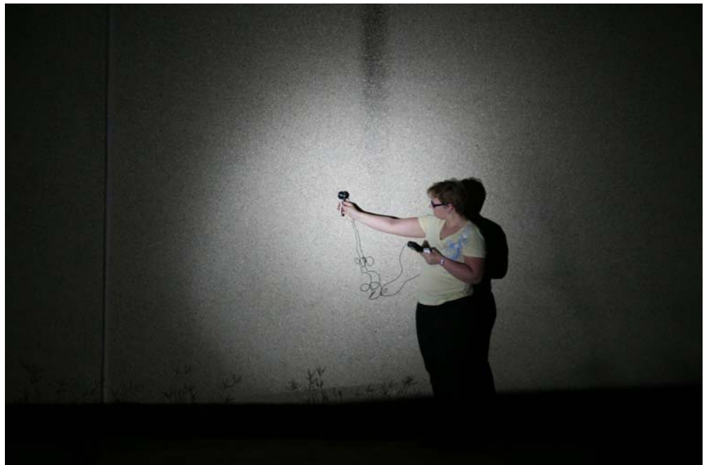
Figure 13 Illuminance measurement of a searchlight.
