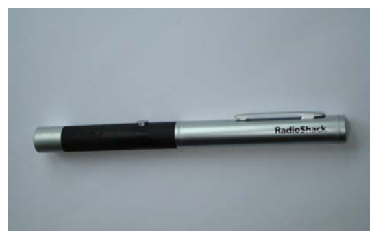
Figure 10 The green laser pointer (Radio Shack, 532 nm).
