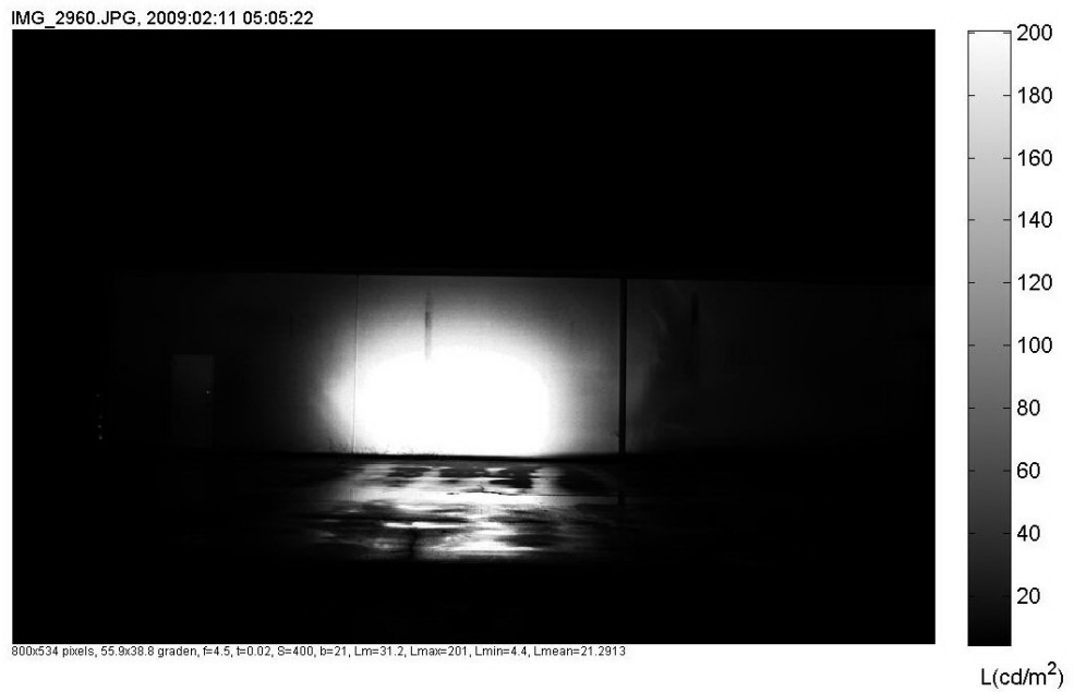
Figure 17 The luminance distribution of the Dominator projected onto a wall at a distance of 100 meter.
